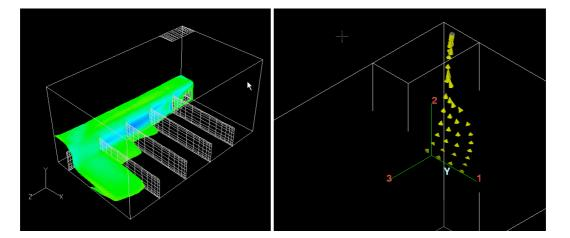
Figure 2: Dynamic interactive 3D visualization of airflow in a livestock building. The CFD (Computational Fluid Dynamics) simulation results were displayed and analyzed with the visualization software VU (Pic and Ozell) in a panorama and a six-sided CAVE environment at VR Media Lab, Aalborg University. (The VU system was launched in 1993 and adapted for VR environments 1998.) From (Svidt et al., 2001)
