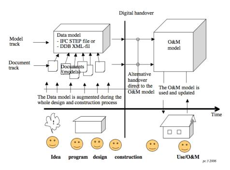
Figure 6: The newly released, January 2007, Danish digital construction requirements let public clients put requirements on the content of the digital models of the building handed over to the client after finalised construction. (DDB, 2006). From (Christiansson, 2007)
