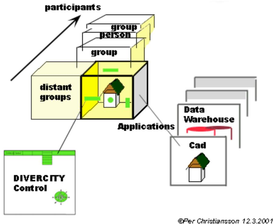
Figure10 Principal Virtual Workspace (VW) layout with 'dimensions' and 'artefacts'. The design object is the Virtual Building (VB). From the DIVERCITY project (Christiansson et.al. 2001)
