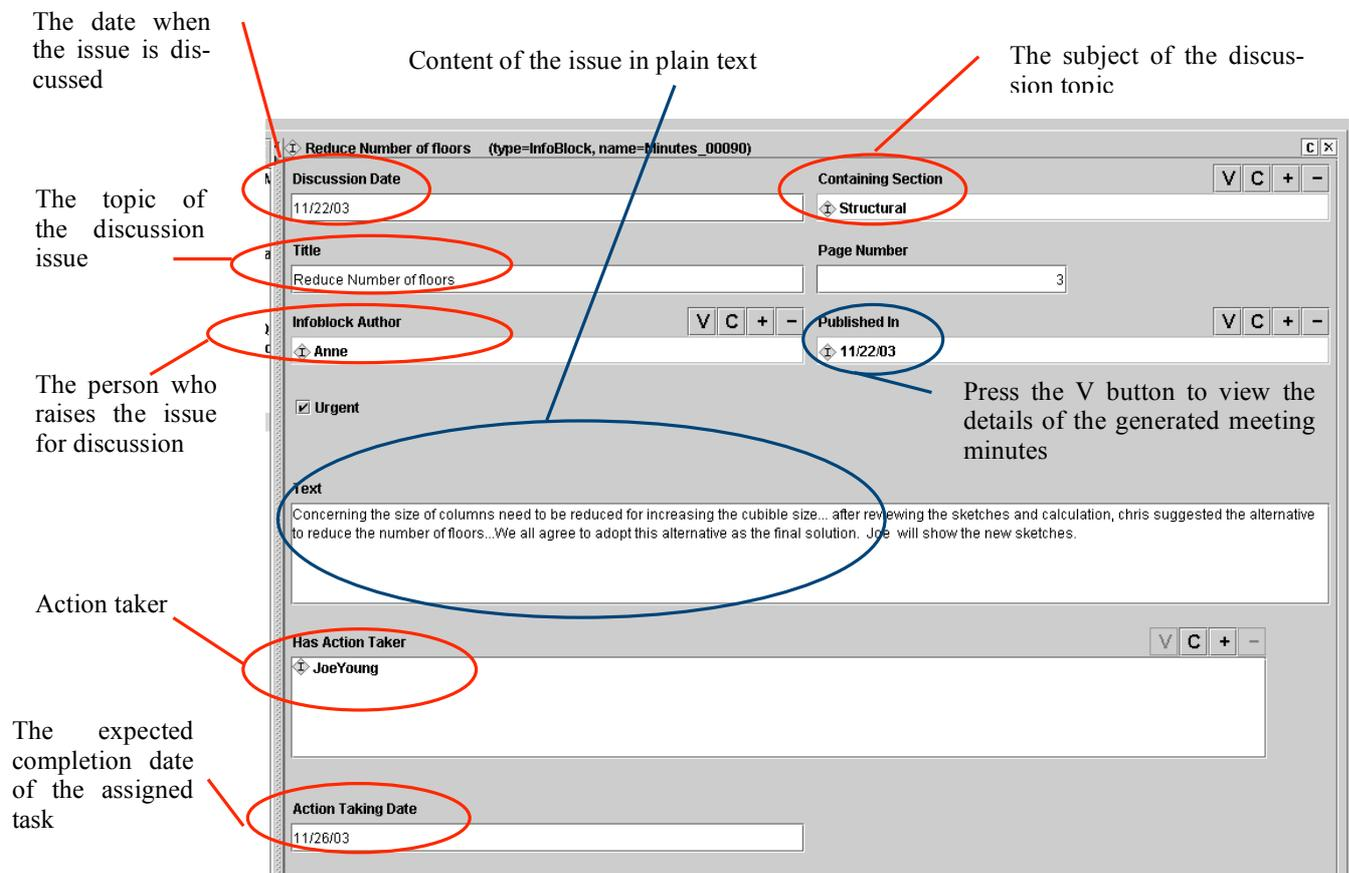
Figure 3. The form filling user interface of the prototype
