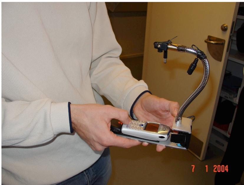
Figure 4 Ericsson T68i Mobile phone mounted on video stand for capture of mobile phone keyboard and screen. The video camera is wirelessly connected to video recording device.
