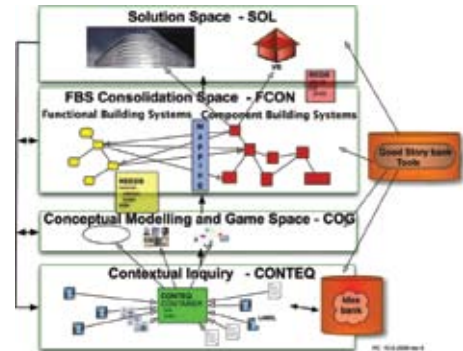
Figure 1. The four design spaces in the Virtual Innovation in design Method, VIC-MET. From (Christiansson et al. 2009a).
